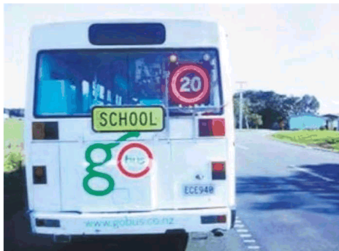
Photograph 3: Bus Mounted Sign – Illuminated 20 kph Sign
