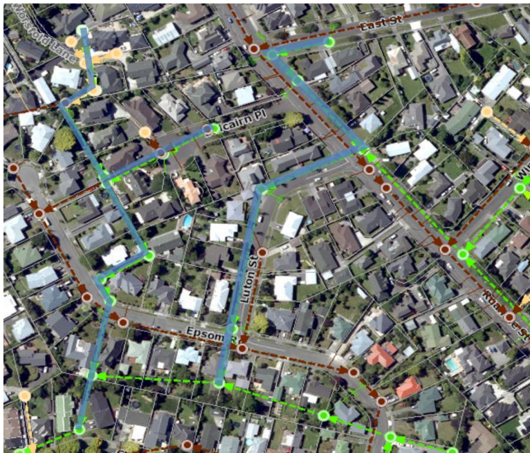
Figure 5 –Proposed Sections for CCTV Inspection 20/21 within Churchill Basin
