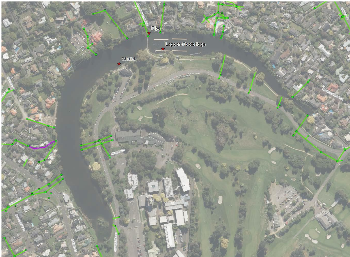
Figure 2 - Existing Stormwater Discharge Locations to Hokowhitu Lagoon.
