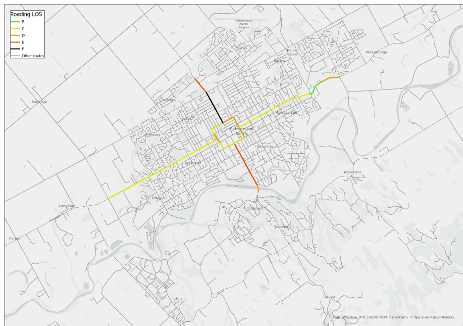
Figure 6-6: Current LOS on general traffic priority network
