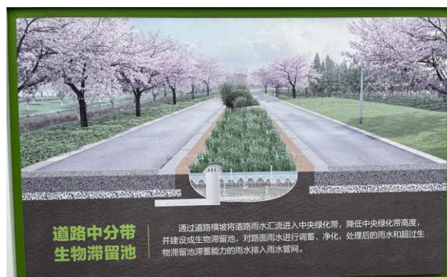
Figure 25- example of sponge city engineering with rain gardens and sensitive planting
