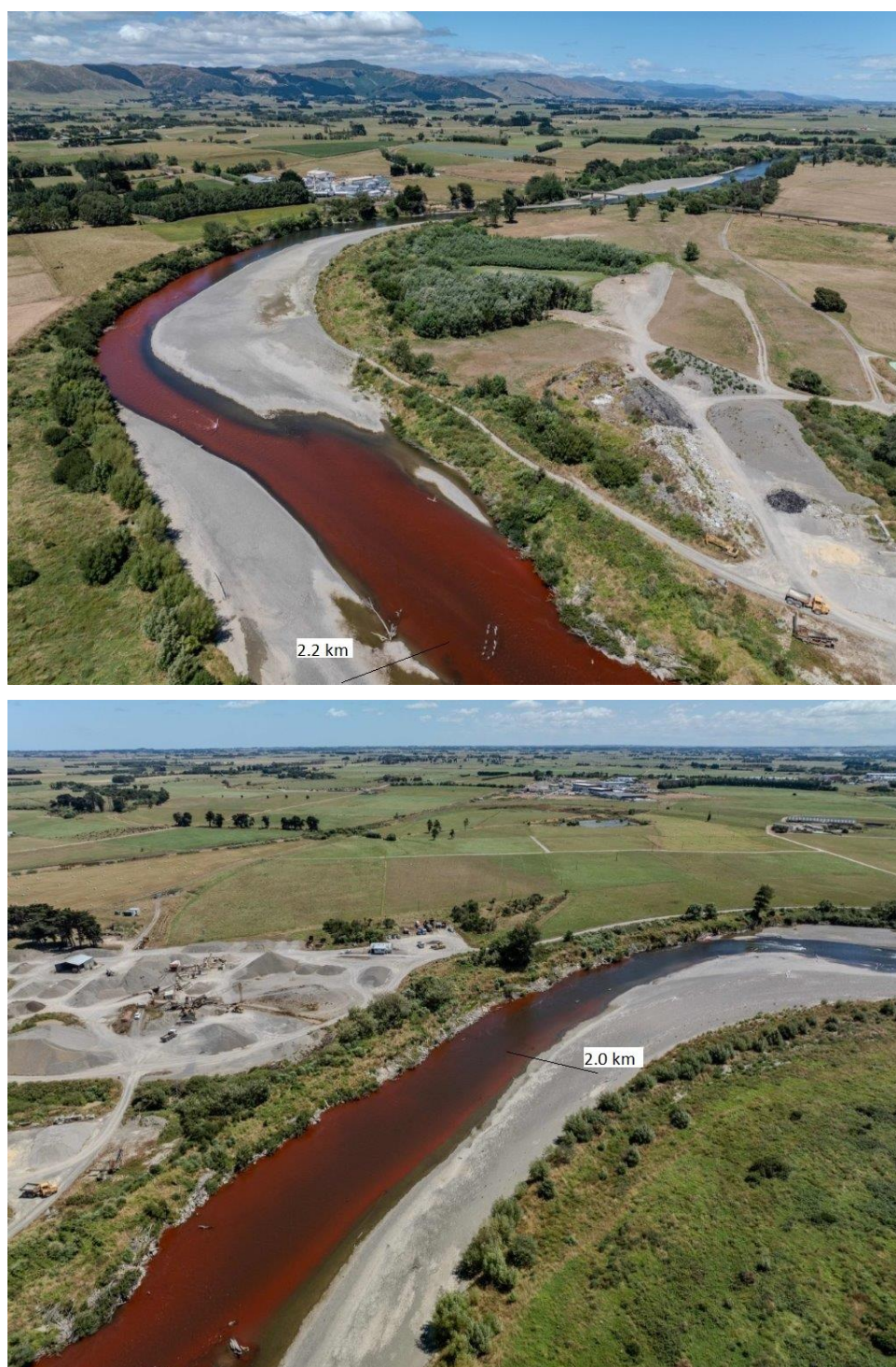
Figure 3.6: Manawatū Longburn facing upstream after dye release from the 1.8km mark (25/1/2024). There is close to full mixing by 200m downstream of the dye release (2.0 km mark). Photos were taken about 15-minutes after the dye release.
