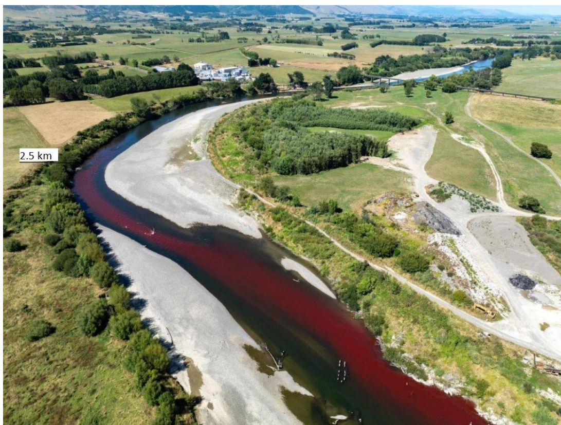
Figure 3.10: Manawatū River at Longburn facing downstream. Dye released at 1.91km downstream of Mangaone on 12/2/2024 resulted in full mixing at the 2.5 km mark.
