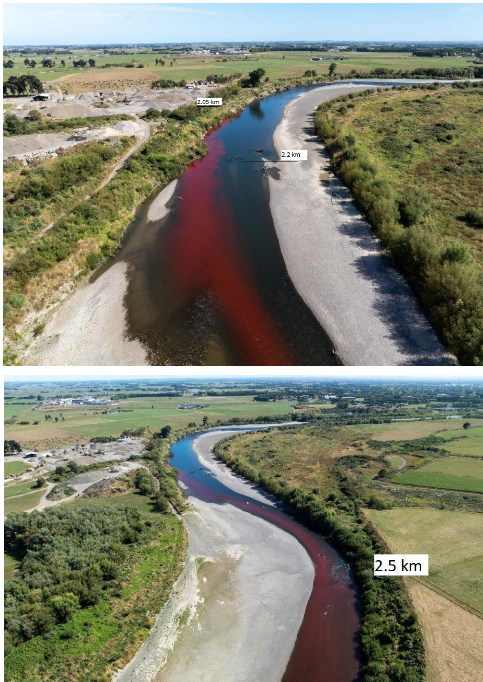
Figure 3.12: Manawatū River at Longburn facing upstream towards the dye release site at the 2.05km mark (upper), and the location of full mixing at the 2.5 km mark (lower).
