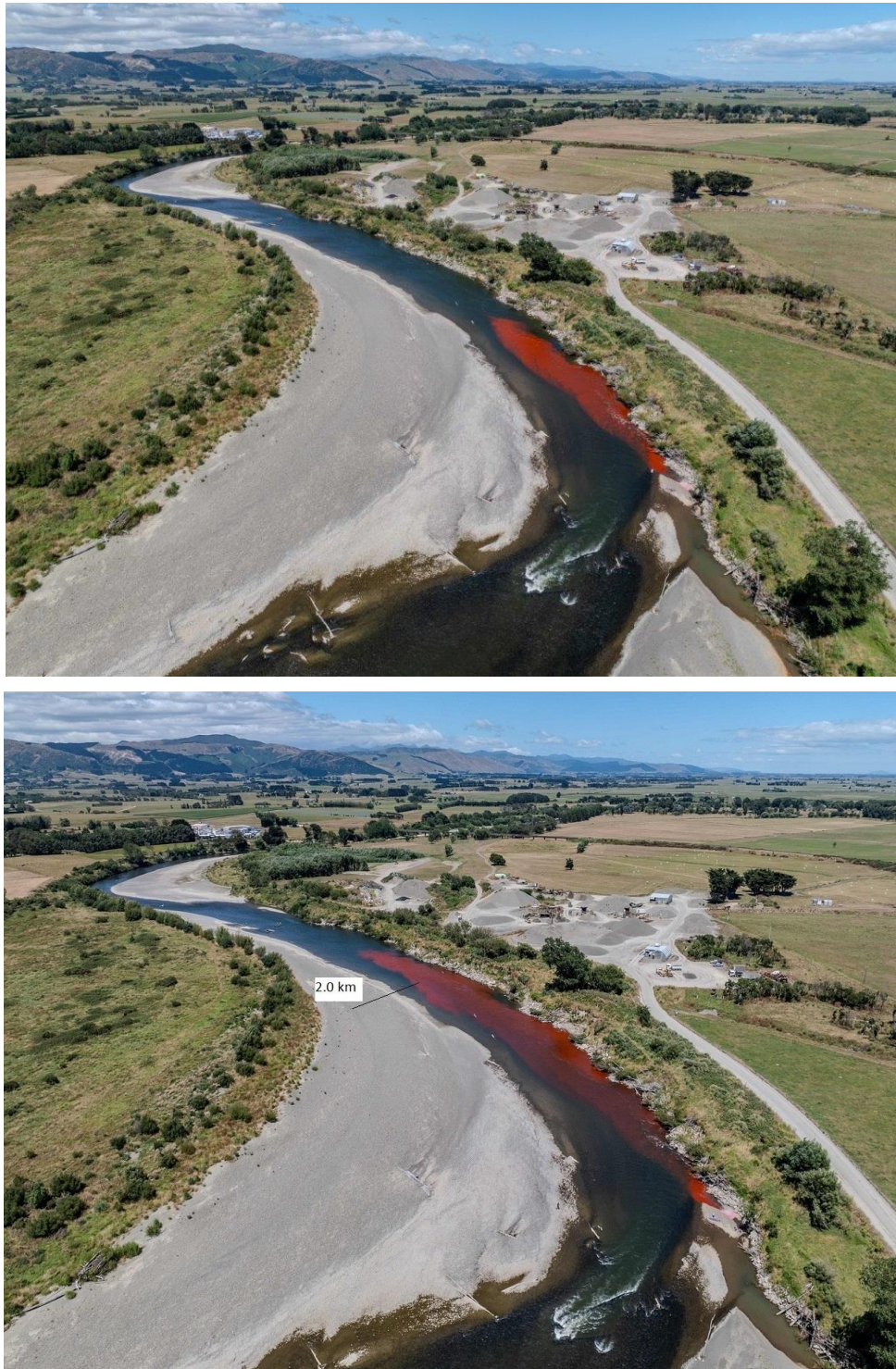
Figure 3.5: Manawatū Longburn facing downstream after dye release from the location 1.8km downstream of Mangaone (25/1/2024). The top photo shows a small promontory at the 1.86km mark directing the current leftward. Both photos are taken within 5 minutes of the dye release.
