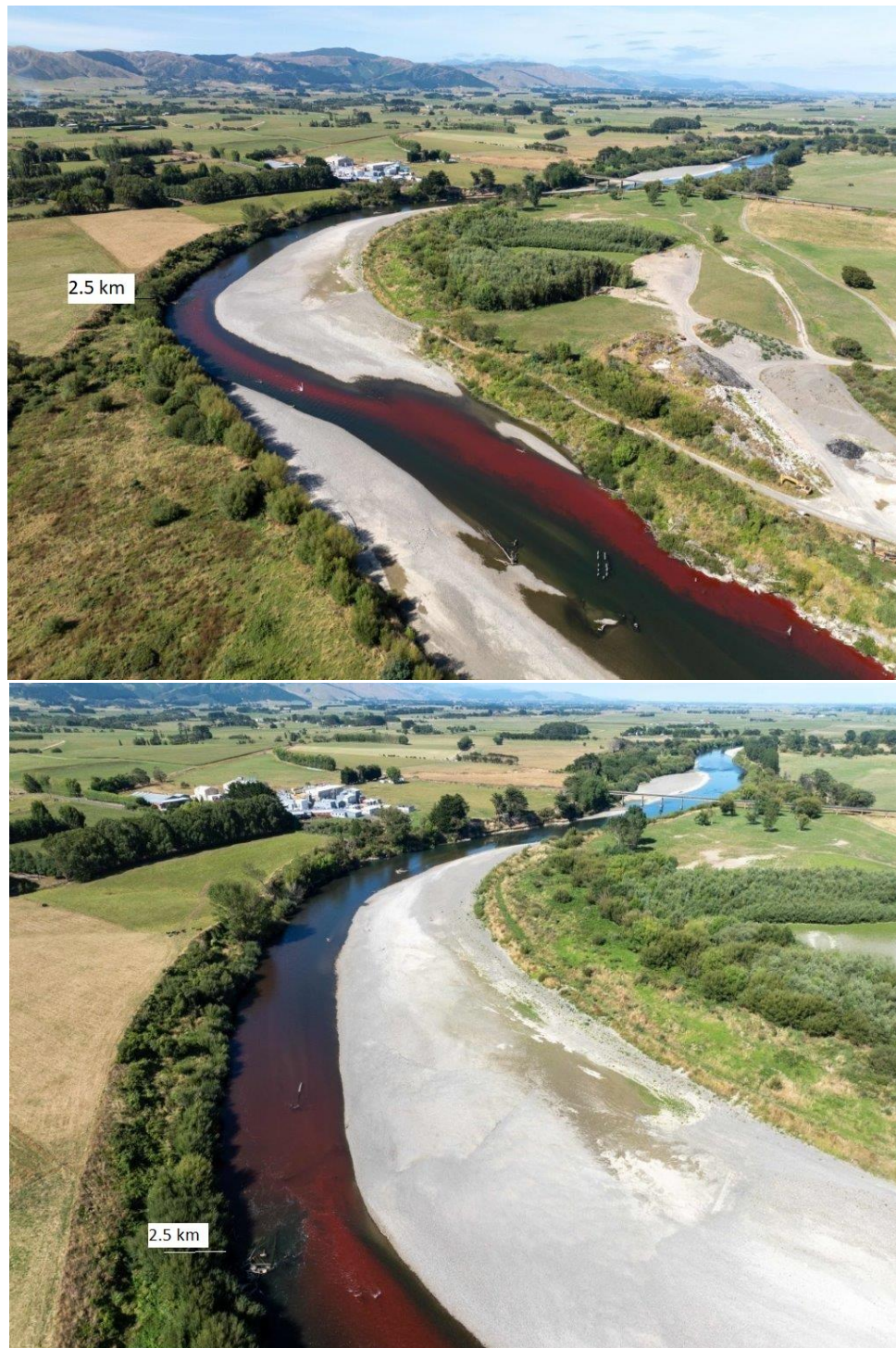
Figure 3.13: Manawatū River at Longburn facing downstream. Dye released at 2.05km downstream of Mangaone on 12/2/2024 resulted in full mixing at the 2.5 km mark.
