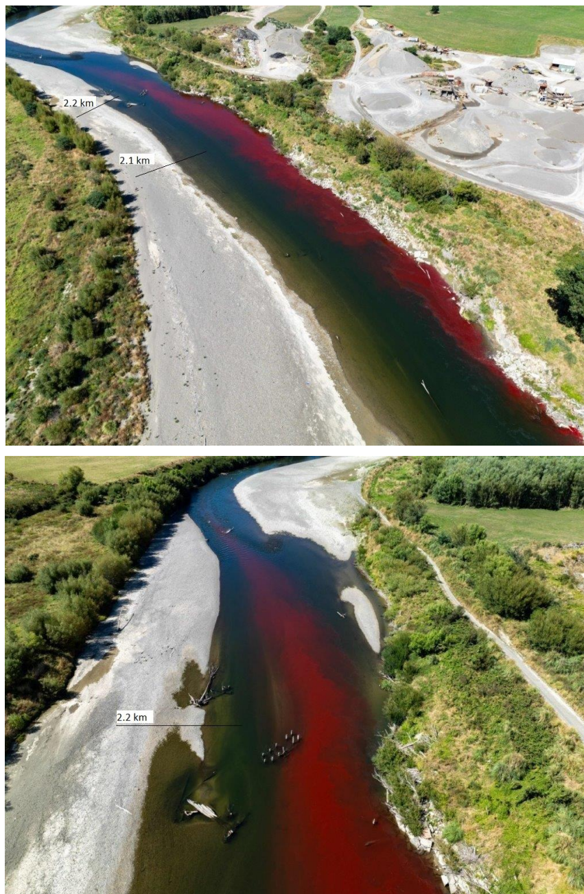
Figure 3.9: Manawatū River at Longburn facing downstream after dye release on 12/2/2024 from the location 1.91km downstream of Mangaone.
