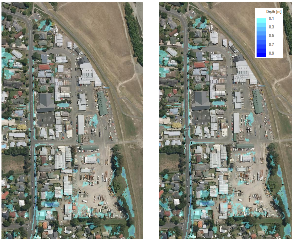
Figure 9: TUFLOW maximum ponding depths for 2% +CC and 1% AEP +CC rainfall events
