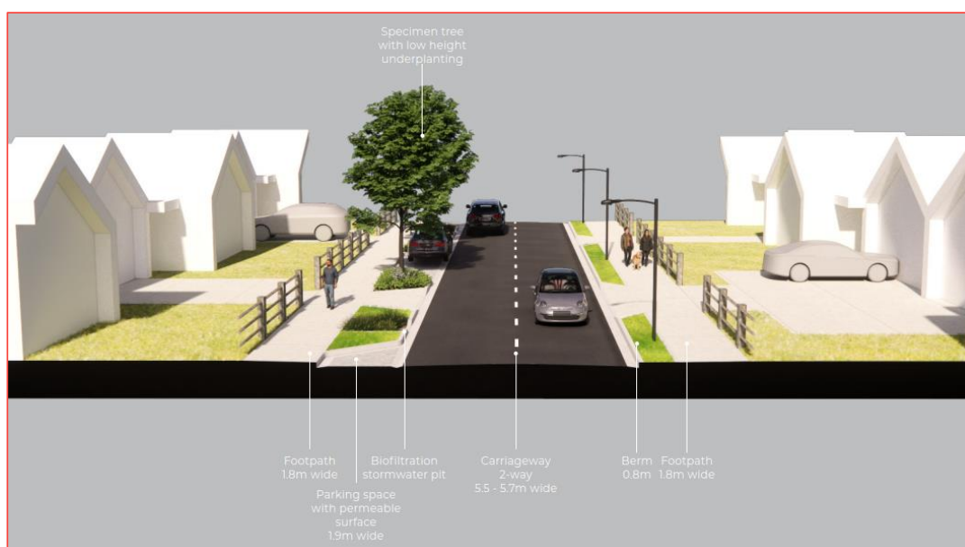
Figure 4-7: Indicative Cross Section Arrangement for a 13m Roading Corridor
