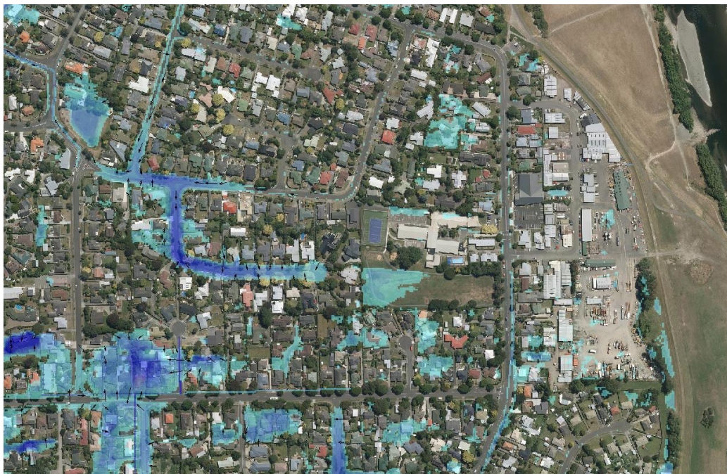
Figure 10: TUFLOW maximum ponding depths for 10% AEP +CC rainfall event
