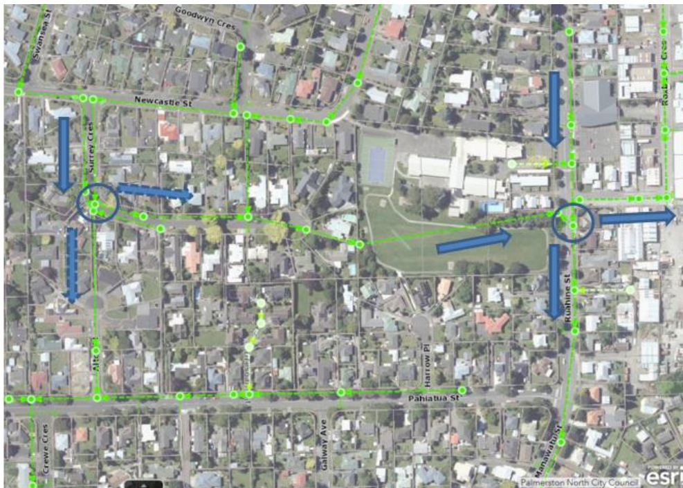
Figure 4: Flow splits (circled in blue) and general flow direction (split flows as dashed arrows)
