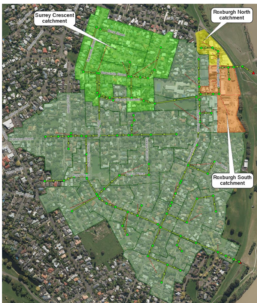
Figure 5: Overview of PCSWMM model of existing network and subcatchments
